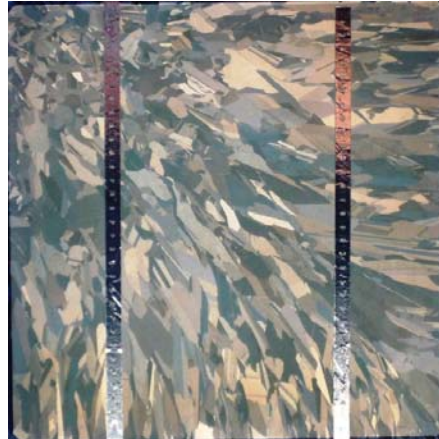
Fig. 1: photo of the microstructure of a polycrystalline Silicon solar cell [2].
